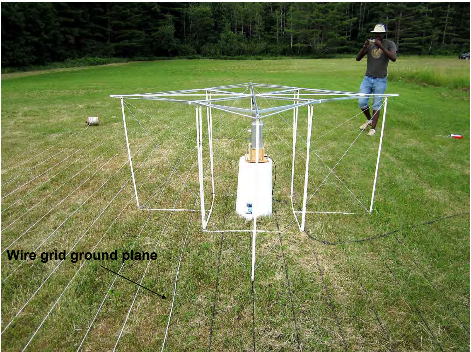
EDGES-2 test of absolute calibration at West Forks, ME
