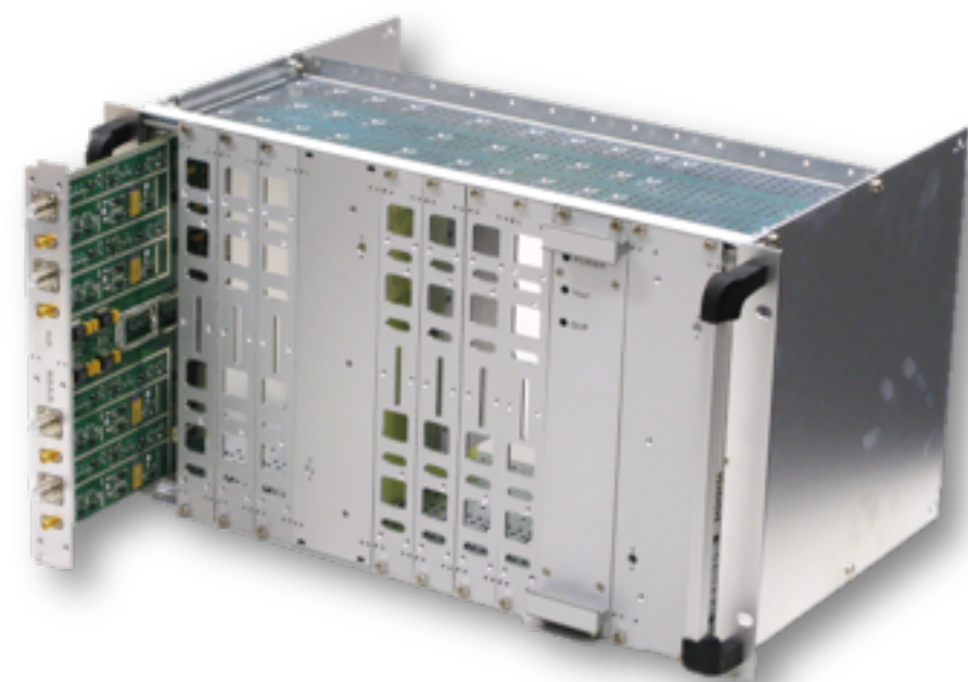
Rack for 8 downconverter boards
