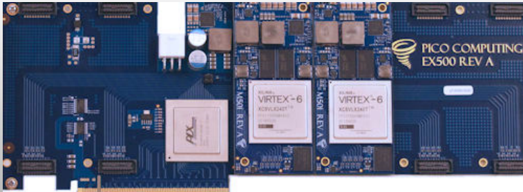
EX-500 backplane with two M-501 FPGA modules installed
