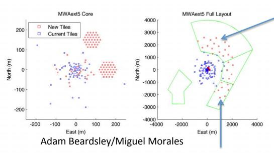
New tiles serviced by independent power systems (solar/batteries)
