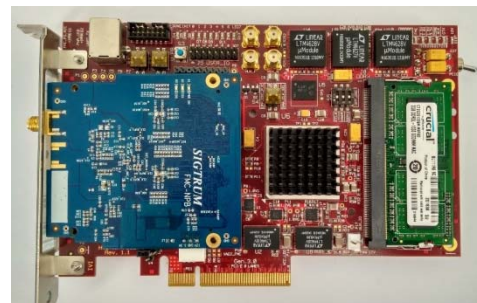
FFTS spectrometer (BW=5GHz, \Delta f=76\text{kHz} )
